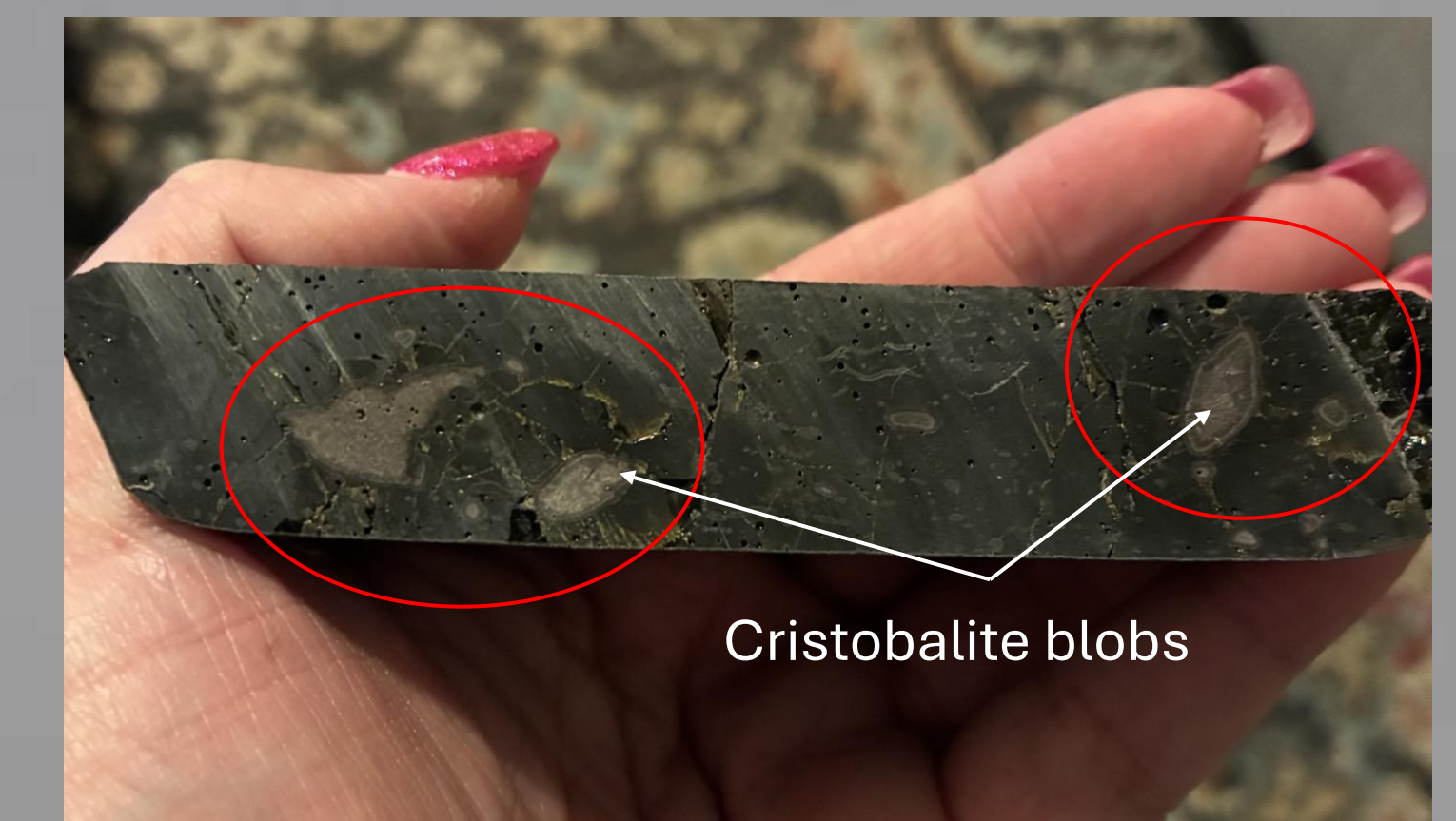
Figure 7. Cristobalite “blobs” in cast CSM-LHT-1 material. Cracks (dark lines) originate from these silica-rich regions, reducing structural integrity post-cooling
